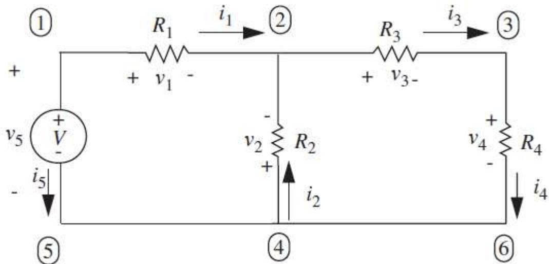
For the above circuit, (1-5) are branch, (6-7) are KVL, (8-10) are KCL equations. Unknowns are  $v_1, v_2, v_3, v_4, v_5, i_1, i_2, i_3, i_4, i_5$  and known voltage is  $V$ .
